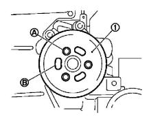
Never install mounting bolts (A) to oblong holes (B). - Water pump pulley (1)
