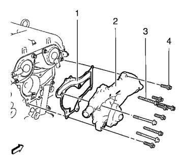
2. Install the water pump (2) and a NEW water pump gasket (1).
